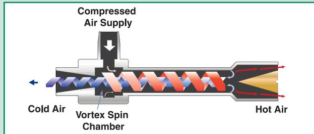
The Mini Cooler incorporates a vortex tube to convert a small amount of compressed air into two low pressure streams, one moving within the other in opposite directions (see page 134). The two airstreams exchange heat, producing cold air from one end of the tube and hot air from the other. A flexible hose directs the cold airstream at the surface to be cooled.
