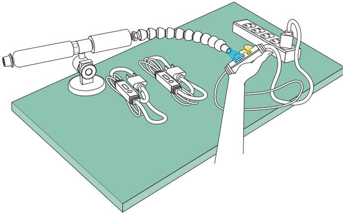
**The Problem:** A manufacturer of electrical heat tapes had a problem testing thermostats for accuracy. The heat tape is supposed to switch on when the outdoor temperature dips below 40°F to prevent pipes from freezing or ice from building up on a roof's edge. The liquid-tight thermostat of every tape had to be dipped into a bowl of ice water (thermometer checked at 36°F (2°C)) to make sure the
